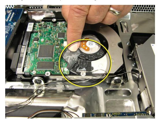
6. Connect the other end of the temperature sensor cable to the logic board.
